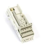
The TU811V1 is a 8 channel 250 V compact module termination unit (MTU) for the S800 I/O. The MTU is a passive unit used for connection of the field wiring to the I/O modules. It also contains a part of the ModuleBus.
