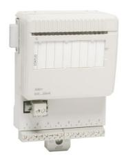
The Al801 Analog Input Module has 8 channels for current input. The current input is able to handle a short circuit to the transmitter supply at least 30 V d.c without damage.
