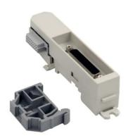
The TB805 ModuleBus Cable Adaptor is used together with TB806 and TK801V0xx to extend the ModuleBus. Using this extension I/O modules on the same electrical ModuleBus can be mounted on different DIN rails.
